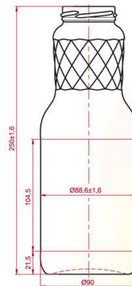
JUICE 1000 Filling capacity 1000ml Brimful capacity 1050 ± 15ml Weight - 440 gr Finish- "TO-53"
